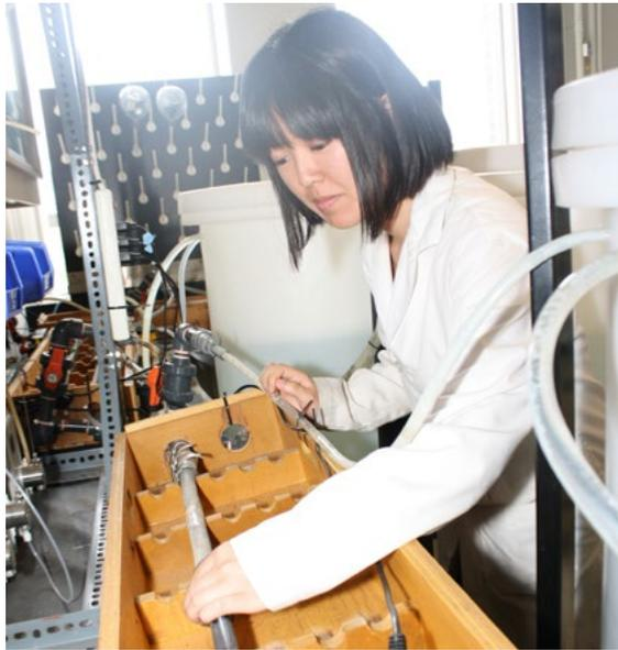
we looked at sodium silicate,” said Payne. “Sodium silicates’ corrosion inhibitor properties have been known since the 1920s, but the funny thing is that no one really knows exactly how they work. So we compared it to the performance of phosphate-based inhibitors to try to understand more about this corrosion inhibitor.”
